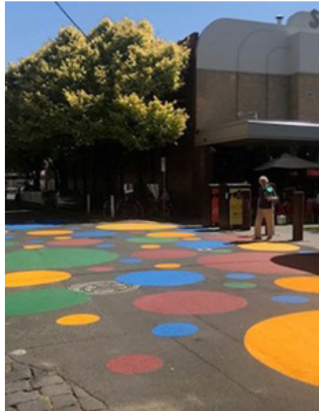
Stencilled paintwork to Devon Place to slow traffic flows and support wayfinding and feelings of activation.
